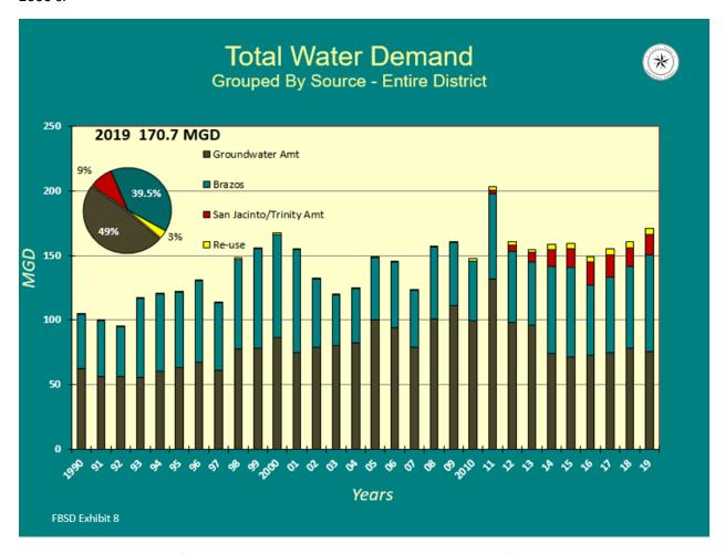
**Figure 10**: Total water use for District, in million gallons per day, by source water, from 1990 to 2019. The reported total water use for the District in 2019 was 170.7 MGD.
