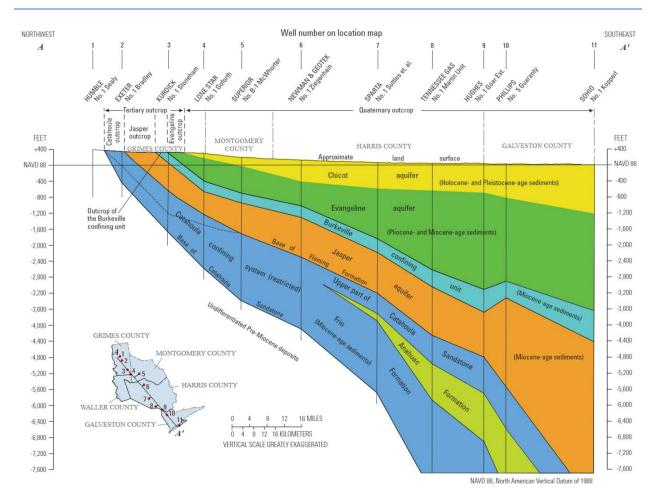
**Figure 1.** Hydrogeologic section of the Gulf Coast aquifer system in Harris and adjacent counties, Texas (Kasmarek, 2013).
