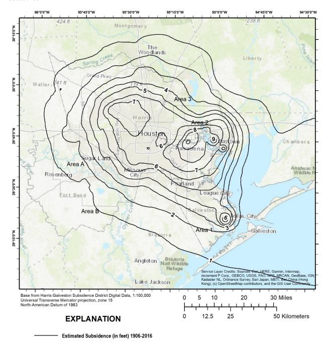
**Figure 17**: Estimated subsidence from 1906 to 2016 using measured land surface elevation change at benchmarks surveyed in 2000 and estimated annual subsidence rates from 2011 to 2016, assuming a constant rate of subsidence from 2010 to 2016.
