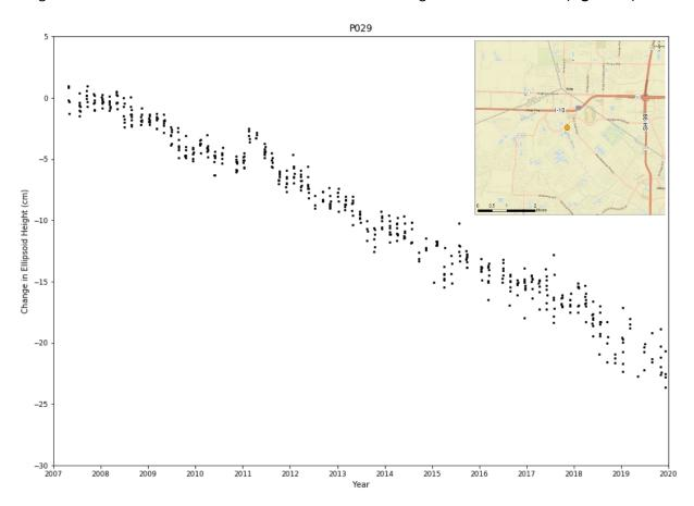
**Figure 14**: Period of record plot for P029 located in Katy, Texas, 2007 to 2019. This site measured 21.52 cm of subsidence over 12 years and the annual subsidence rate is 1.95 cm per year. The inset map shows the location of P029, the orange circle southwest of the intersection between I-10 and SH-99.
