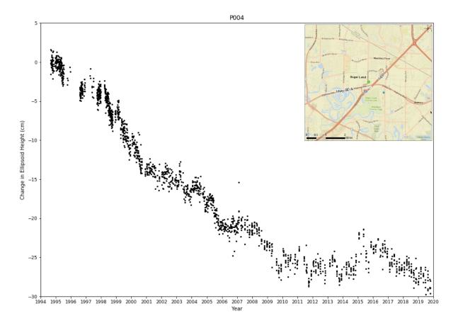
**Figure 15:** Period of record plot for P004 located in Sugar Land, Texas, 1994 to 2019. This site measured 28.41 cm of subsidence over 25 years and the annual subsidence rate is 1.24 cm per year. The inset map shows the location of P004, the green circle northwest of the intersection between I-69 and Highway 90A.
