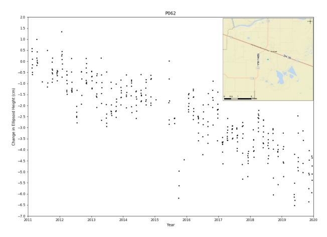
**Figure 16**: Period of record plot for P062 located in Orchard, Texas, 2011 to 2019. This site measured 5.07 cm of subsidence over eight years and the annual subsidence rate is 0.62 cm per year. The inset map shows the location of P062, the blue circle southeast of the intersection between FM-1489 and SH-36.
