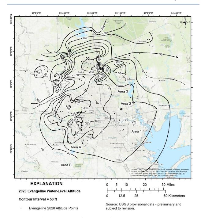
**Figure 11**: Altitude of the potentiometric surface determined from water-levels measured in tightly cased wells screened in the Evangeline aquifer, Houston region, Texas, 2020 (Source: USGS provisional data – preliminary and subject to change).
